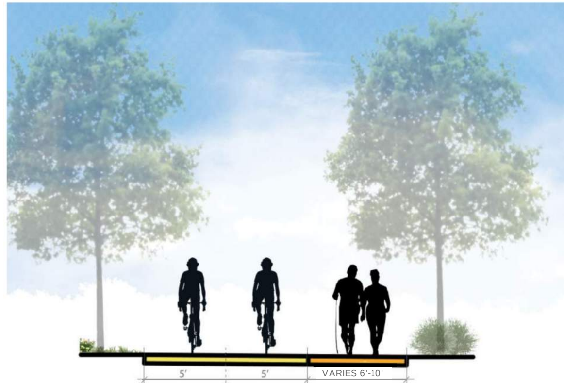
TYPICAL SHARED USE PATH CROSS-SECTION
